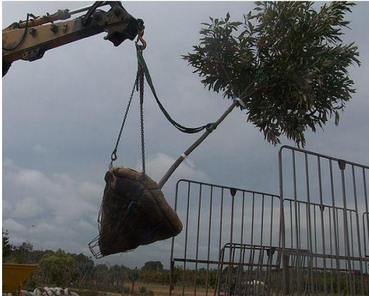
Lifting the tree: Note the saver sling attached with no weight being taken by the sling. This method will get the tree to the hole without any damage being caused by the machinery. The lifting lugs on the cage are taking all the weight.
